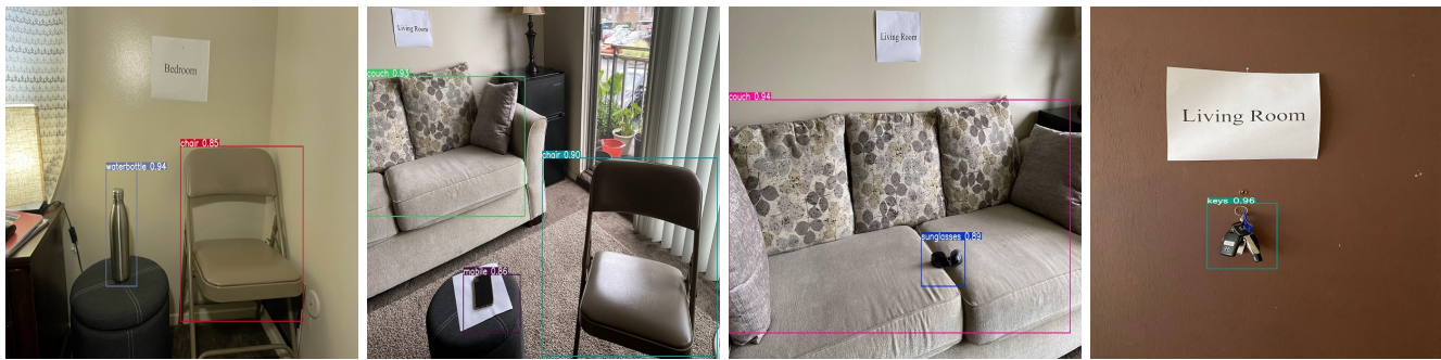
Fig. 3. a) Target object is at the right side of the Reference object b) Multiple reference object detected c) Target object is on the Reference object d) Target object detected without Reference
