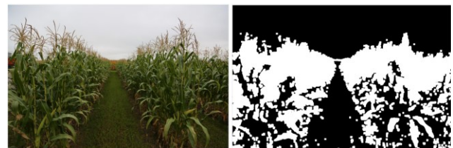
Figure 11: Hough transform preprocessing binarization showing crop and grass separation with the sky seen as the same type of area as the grass
