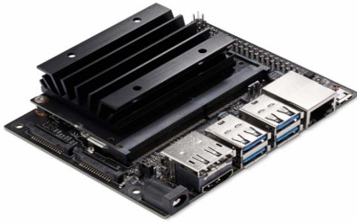
Fig. 8. NVIDIA Jetson Nano [21]
