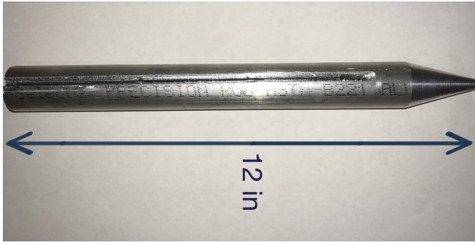
Fig. 3: Aluminum rod, to be inserted in tree trunk horizontally along a radius.
