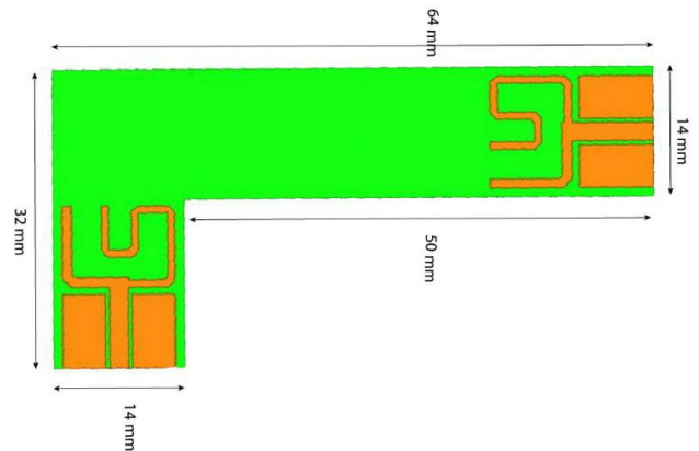
Fig. 8. Schematic for the 2 \times 1 dual band MIMO antenna.
