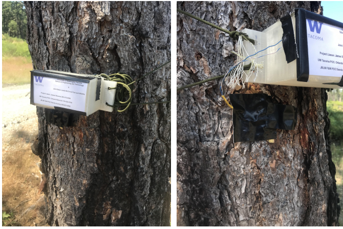
Fig. 2: TEG devices installed on tree trunks in Washington State
