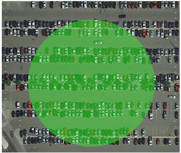
Fig. 16. Coverage area an AP can expect with the tested range of 160ft.
