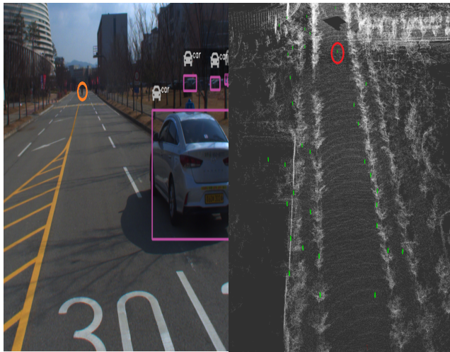
Fig. 6. In part-a showing the camera image while in part-b is the radar data of detection and tracking on real environment.
