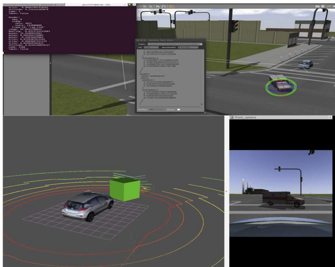
Figure 6 : RADAR sensor view in Rviz
