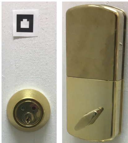
Fig. 6. MRCP Smart Lock Exterior Side (Left) and Interior Side (Right).
