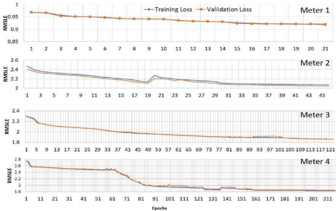
Fig. 4: RMSLE versus epochs of the DNN for different meters
