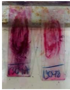
(b) Sample with fuchsin coming from the equipment (left) and uncontaminated fuchsin (right).
