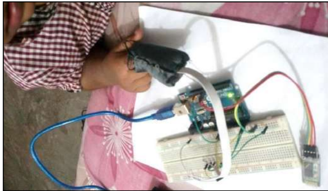
Fig. 4. Application of implemented Oximeter on children that measures SpO 2 (%)
