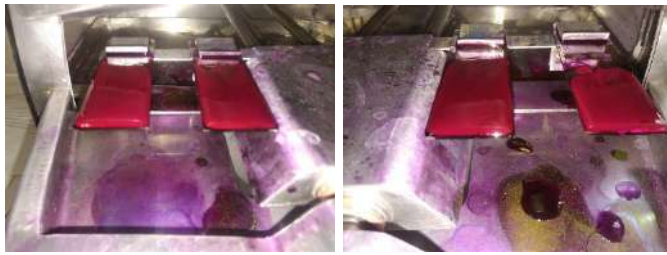
Fig. 14: Fuchsin coating of samples after heating.
