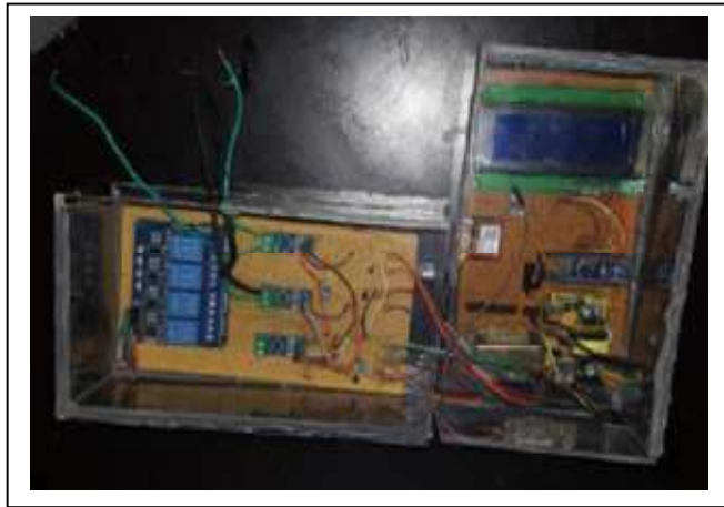
Fig. 5. The developed hardware of the IoT-based metering system
