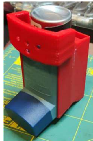
Figure 6. 3-D printed prototype of the final sleeve design model
