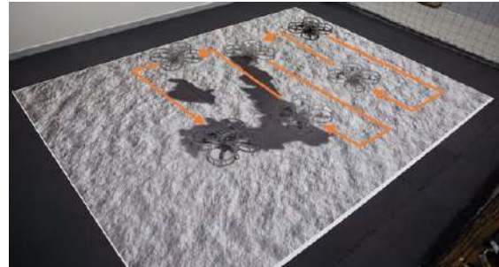
Fig. 4. The drone is flying above an image of an oil spill case in the ocean
