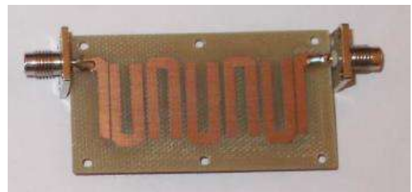
Figure 6: Fabricated fifth-order bandpass filter with FR-4 substrate.
