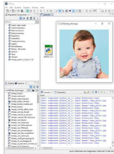
Figure 6. Evaluation of CondenseNeXt on CIFAR-100 dataset when deployed on NXP BlueBox 2.0 using RTMaps Remote Studio 4.8.0 for classifying an image of a baby and outputting the predicted class in RTMaps console.
