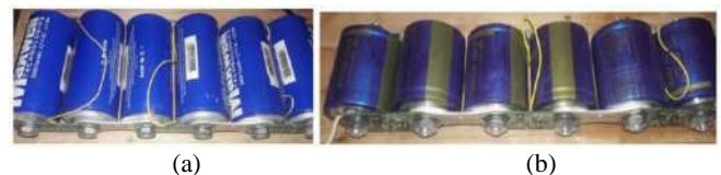
Fig. 4. (a) Supercapacitor bank and (b) hybrid capacitor bank.
